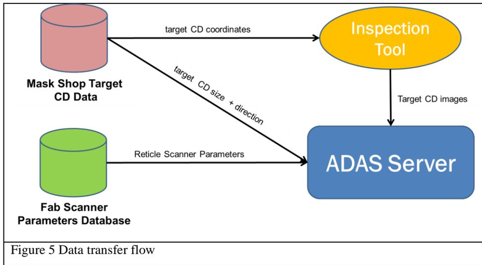
Once the inspection is loaded into the ADAS server, the operator views the target CD image, selects the measurement area, and then selects the “Auto Threshold” button. ADAS then displays the CD target value and orientation, and automatically adjusts the threshold to match the target CD value as seen in Figure 6 below.
