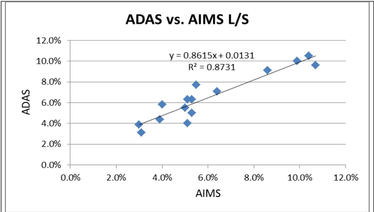
Fig. 9 ADAS vs. AIMS CD percentage error results comparison
