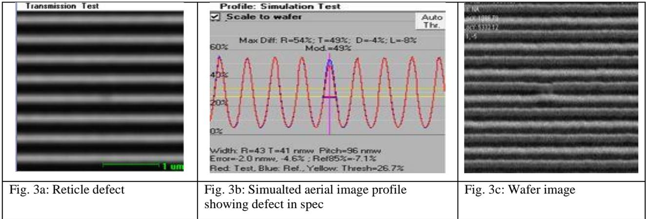
Once simulated with the correct threshold, the defect was correctly simulated to be out of spec (see Figure 4). This shows how important it is to have a proper threshold for simulation. Human errors can cost a lot of time and money and this is the main motivation going forward to have more automated procedures in place.
