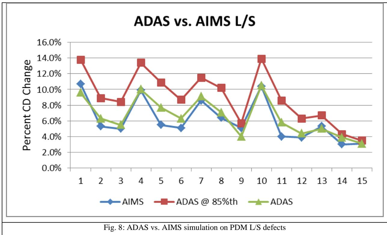
Figure 9 shows a good correlation of percentage CD error between ADAS and AIMS. It's also seen in the graph that ADAS tends to overestimate CD errors, especially on defects measured to be over spec on the AIMS tool.
