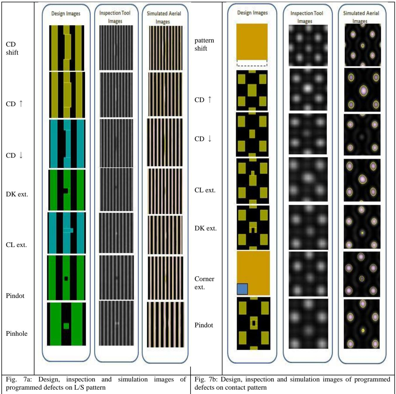
Fig. 7a: Design, inspection and simulation images of programmed defects on L/S pattern
