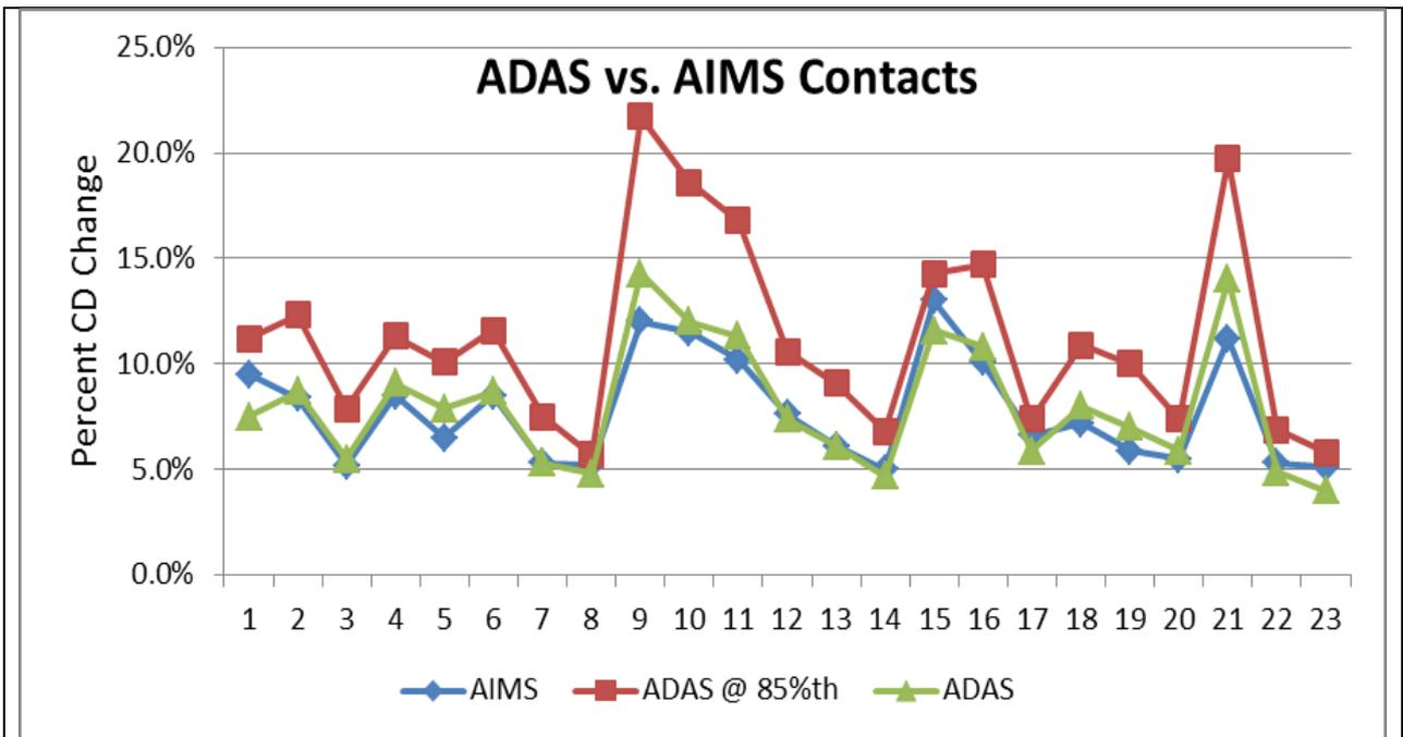
Figure 10: ADAS vs. AIMS simulation on PDM contact pattern defects
