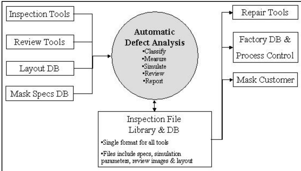
Figure 1: Automatic defect analysis environment
