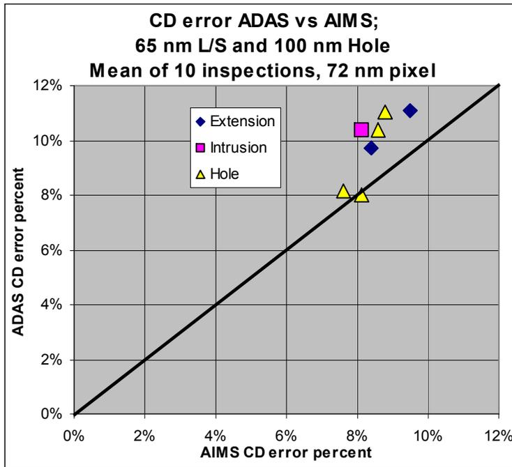
Figure 4: CD error measurement comparison ADAS – AIMS
