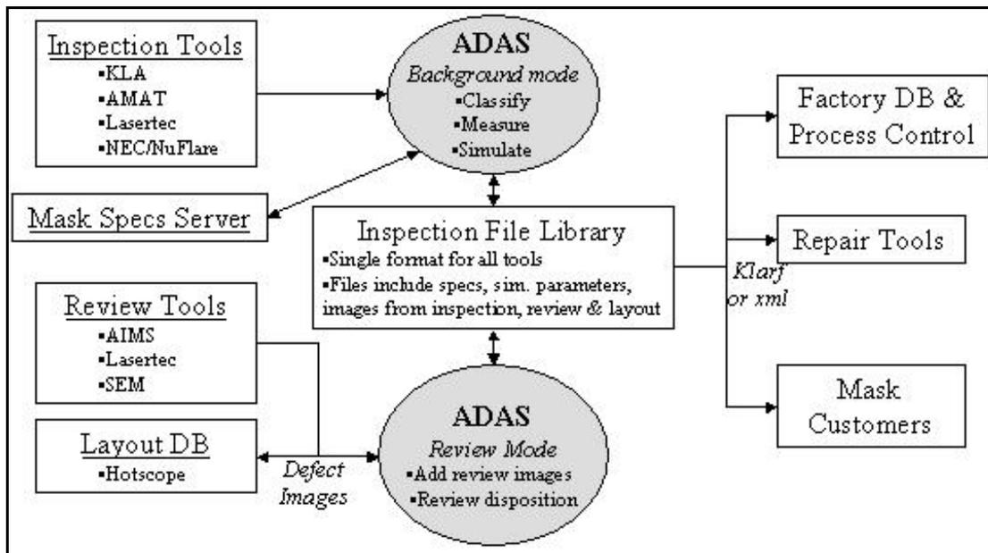
Figure 2: ADAS Inputs and Outputs
